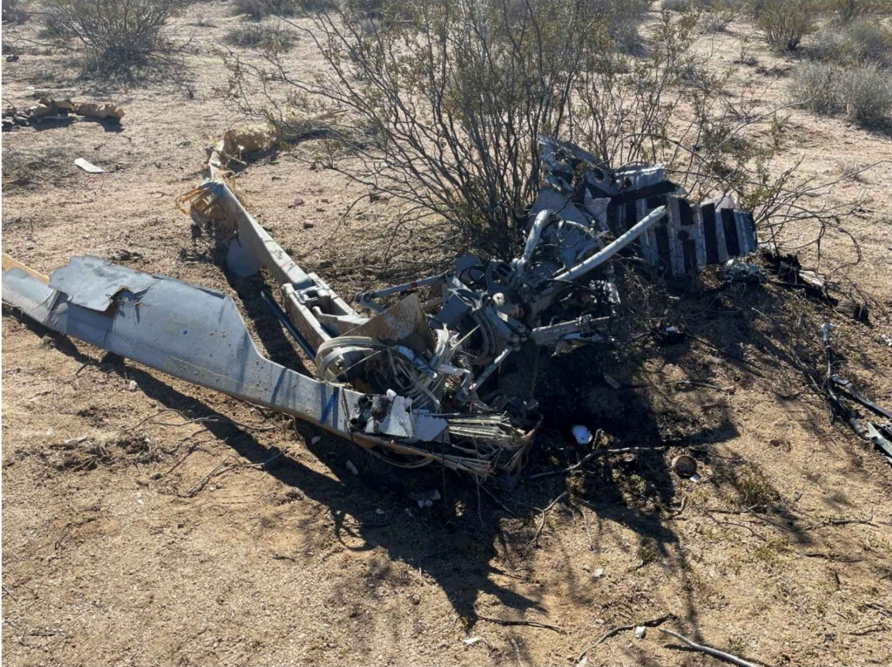
Figure 4. Rotor mast and rotor head.
